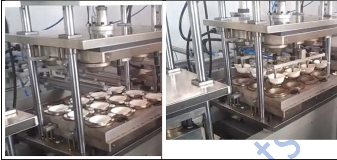
Above photograph shows bowls cured in a compression moulding press being taken out
